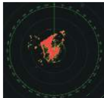
Interference rejector on; interference suppressed
