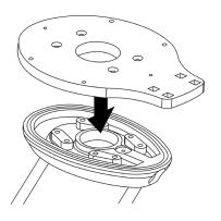
Secure the ADA-F3 with the four bolts using a 3/16" Allen Wrench.
