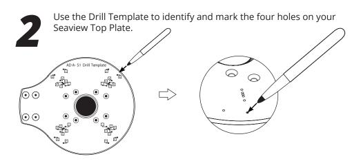
Drill the four marked holes. Be sure to check with your marine electronic manufacturers manual to determine what size drill bit is needed.
