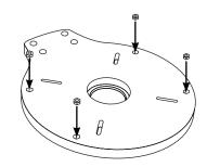
Apply marine adhesive sealant along the lip in the center hole on the adpater plate.
