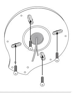
Attach the satellite dome to the adapter plate, and secure with the hardware for your electronics.
